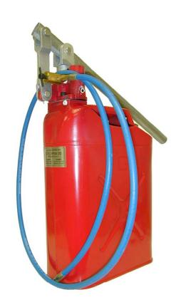
The hand pump is mounted on a 20-litre (5 gallon) metal container and has a rubber core steel braided discharge hose for easy connections and a convenient pressure relief valve. Working pressure up to a maximum of 1000 psi. Discharge stroke volume is 2.29 cu. in or 37.5 ml.
