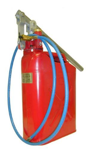
The hand pump is mounted on a 20-litre (5 gallon) metal container. Other features include adjustable pressure settings (1000, 2000 and 3000 psi), rubber core steel braided discharge hose for easy connections, convenient pressure relief valve and a discharge stroke volume of .730 cu. in or 11.96 ml.
