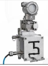
Sliding key back in neutral position. LP, HP side de-blocked. DP is measured. Proximity switch signals: "measurement is integer".
