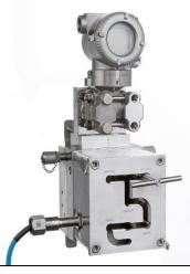
Venting LP side. Key cannot slide to other position before blocking the vent again.
