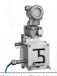
HP side is isolated/blocked. Key cannot go back to neutral position before deblocking HP again. Key can only slide to LP side as long as HP is blocked. Proximity switch signals: "measurement is NOT integer".
