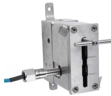
The key has left the neutral position. The first isolate is blocked. The key cannot slide back to the neutral position before the first isolate is de-blocked. The key cannot slide to the second isolate before the first isolate is blocked. Proximity switch (optional) signals: "measurement is NOT INTEGER".
