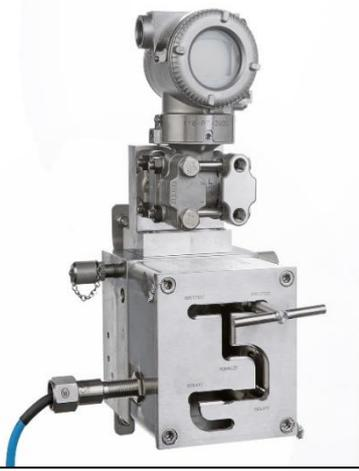
Venting LP side. Key cannot slide to other position before blocking the vent again.
